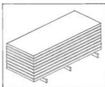
Doors should be protected from dirt and damage but without restricting air circulation.
