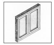
Preglazed and prefinished windows should ideally be fitted into preformed openings and not 'built in' to masonry walls.
