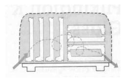
When stored inside a building, windows should be protected from dirt and damage but without restricting air circulation.
