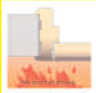
Fire door in action
