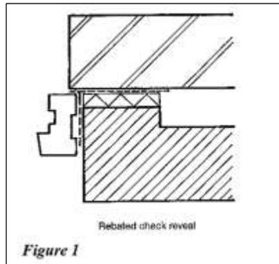
In exposed conditions consideration should be given to using a rebated check reveal (Figure 1)
