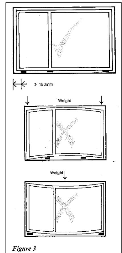
Support for the frame should be such as to prevent distortion and should not damage any protection or finish.
